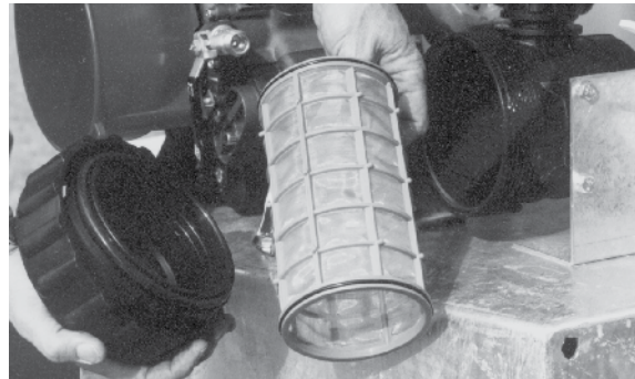
Remove & clean the filter element & components
