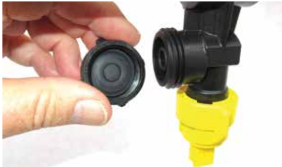
Remove & clean the non-drip diaphragms regularly
