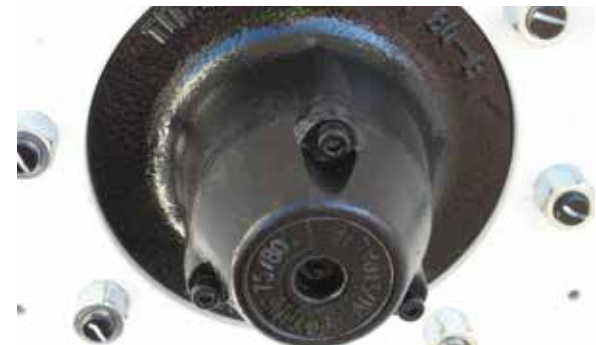
Repack the wheel bearings at 200 hours
