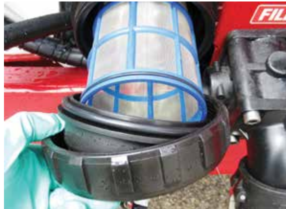
Remove the outer screw and bowl of suction filter
