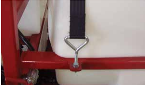
Check the tank straps
