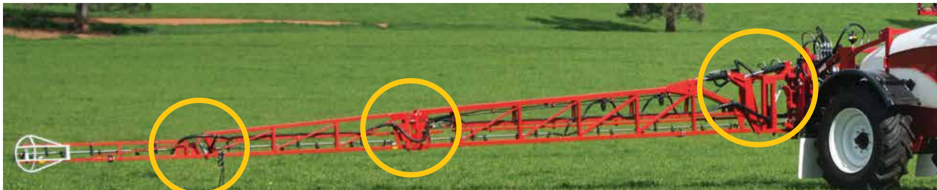
Photo shows main zones of boom adjustment
