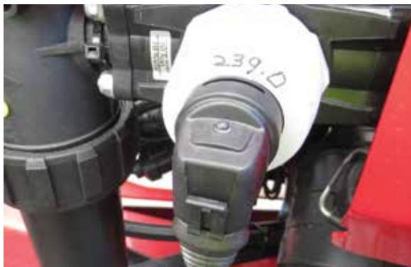
Clean the Flowmeter
