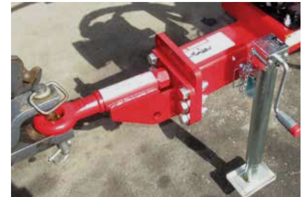
3000 Hitch - 3 bolts per side
