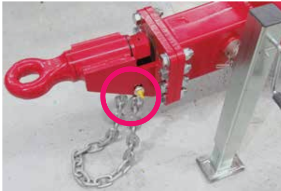
4000 Hitch - 4 bolts per side
