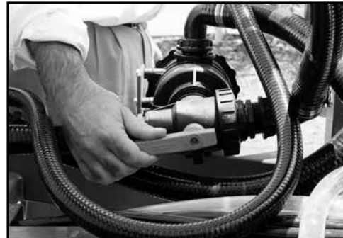
(3) Check the directional valve is from the spray tank.
