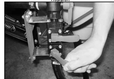
(n) Open the drum rinse valve to rinse the hopper.
