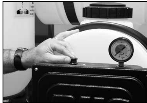
Foam marker adjustment knob & pressure gauge.
