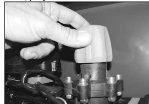
(7) Adjust the manual relief valve.
