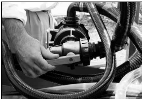
(e) Turn directional valve to source from spray tank
