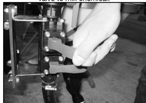
(k) Close hopper lid & open the nozzle rinse valve to mix chemical.
