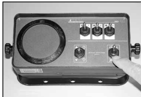
(13) Check and adjust pressure with boom switches ON.
