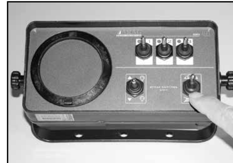
(6) Pressurise the system with the Master Switch in ON position.
