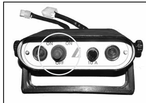
Use the left/right selector switch to send foam to the left or right foam nozzle
