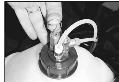
Always release air-pressure in the tank before undoing the cap to refill, and when finished for the day.
