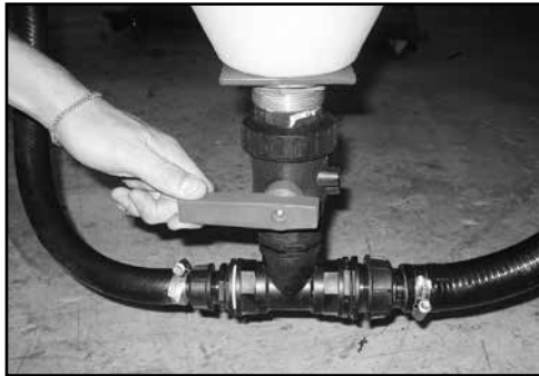
(p) Close transfer valve at the base of the hopper.
