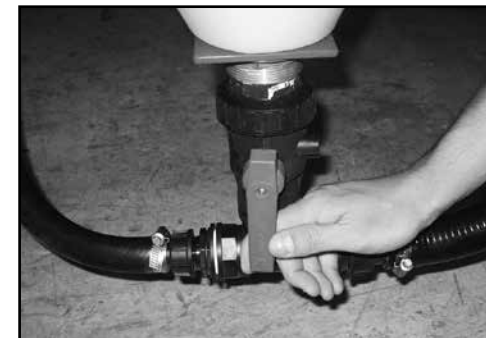
(m & o) Open transfer valve to transfer mixture to the spray tank.
