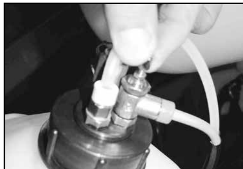
Adjust foam output with the flow-rate regulating valve.
