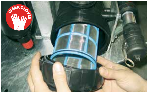
Remove the outer filter screw and bowl
