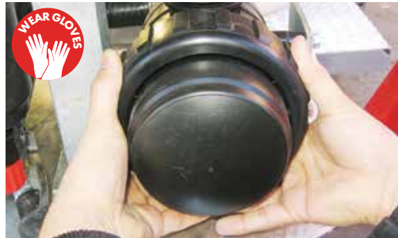
Reassemble and tighten the outer filter screw.
