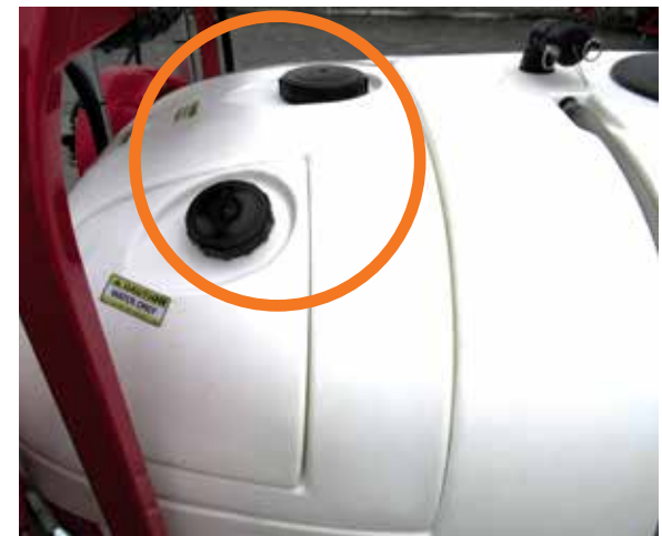
The 2000 model features separate flushing and handwash tanks integrated into the design of the main tank (circled).
