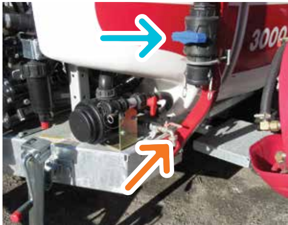
Filling the Main tank can be via the basket or separate / remote fill tap and camlock (see blue arrow). On the 2000 model the camlock is on top of the tank. The freshwater Flushing tank on the 4000 model is
