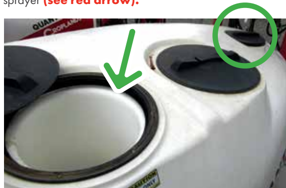
The 2000 model features separate flushing and handwash tanks integrated into the design of the main tank (circled).
