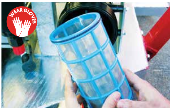
Remove & clean the filter element & components
