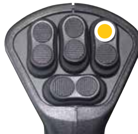
Section RR is turned on/off with SW3
