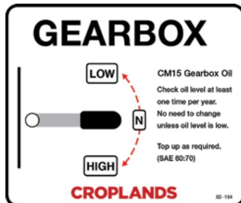
To avoid damage to the gears of the gearbox and to the sprayer unit, **always disengage the PTO drive before operating the gearbox lever / changing gears etc.**
