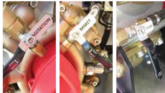
16. Ensure all spray function controls are in the OFF / bypass position.
