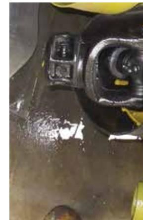
Incorrect hitching of PTO shaft will result in excessive pump vibration.
