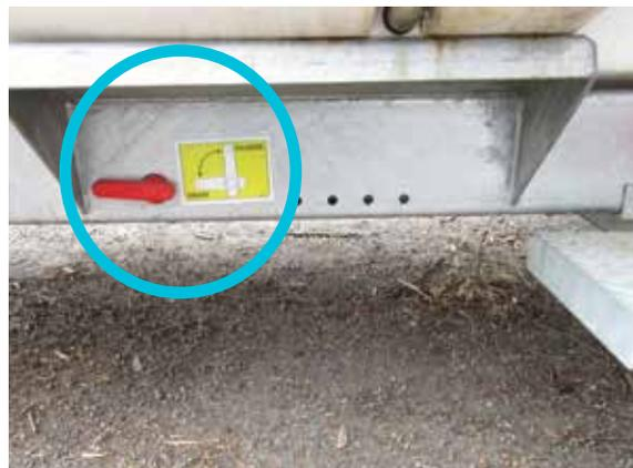
The 4000XL model is fitted with an external flushing fitting via camlock connection. The ball valve can direct flow to fill the flushing tank or to the tank selection valve which can be used to flush the complete plumbing system. **Orange circle.**
