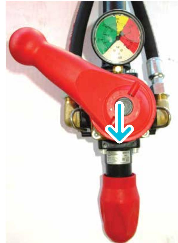
Shown above in the bypass position. Photo to the far left is both booms on.
