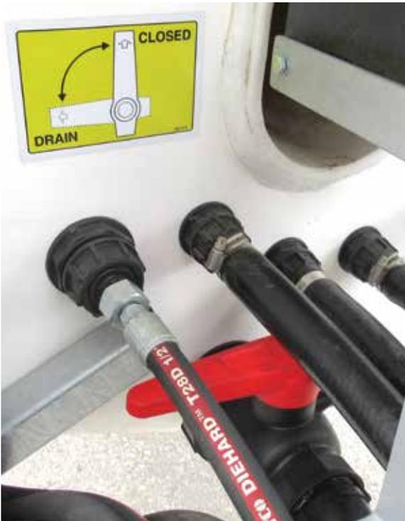
4. Open the Tank Selection valve to the FLUSH position, as shown below (2000 ~ 4000 models).
