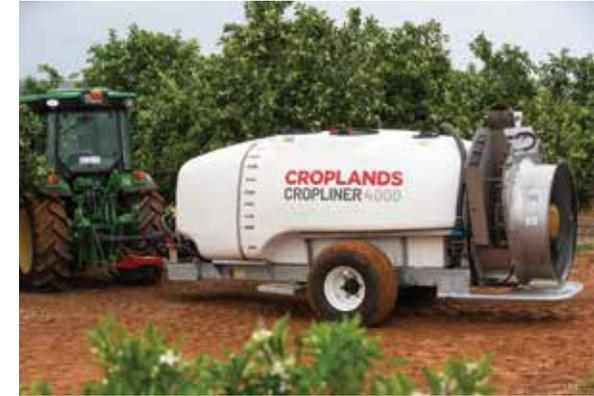
Tractor size / power required is dependent upon a combination of weight (sprayer tank capacity), fan (size and pitch angle setting) and farm conditions (soil and terrain).
