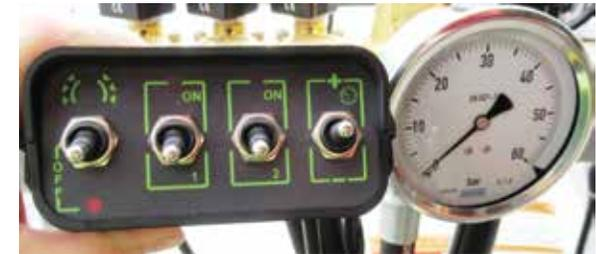
The master switch has 2 off positions. The fully down OFF position (shown above) will draw power (light is on). The bypass (dump) valve is open and there will be no pressure.
