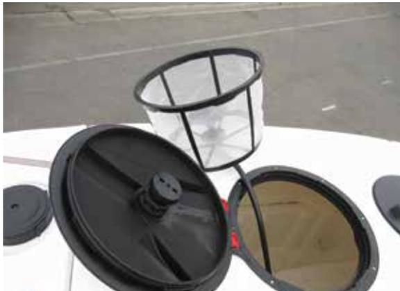
Filling the main tank can be via the basket or via a remote fill tap and camlock at the rear of the sprayer. The fill camlock can be seen on top of the sprayer. (see Green arrow).
