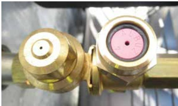
**Fieni 820 ~ 920 DSV Fan, as factory fitted "standard", AlbuZ ATi Hollow Cone Nozzles.**
