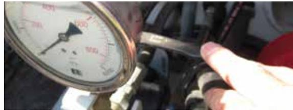
The tap on the back of the pressure gauge is used to relieve sediment trapped in the gauge line. Use at least daily or more often if the water source isn't clean, and whenever freshwater flushing.
