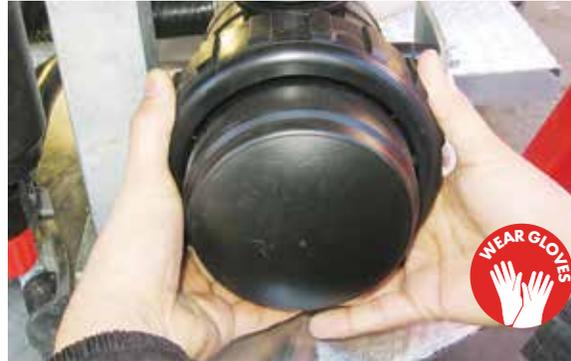
Reassemble and tighten the outer filter screw.
