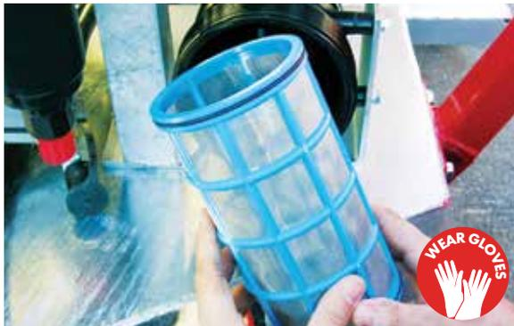
Remove & clean the filter element & components
