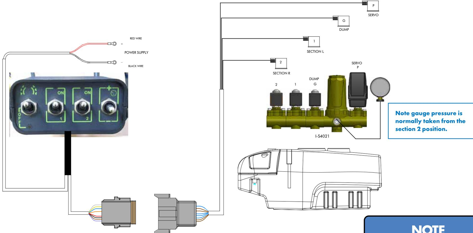
Note gauge pressure is normally taken from the section 2 position.
