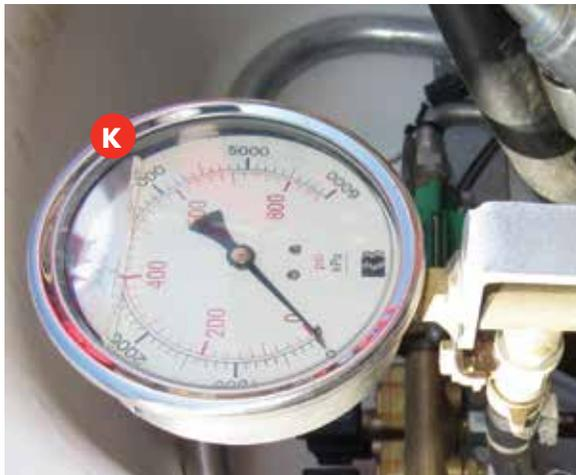
K. The main pressure gauge is also connected to the spray manifold.
