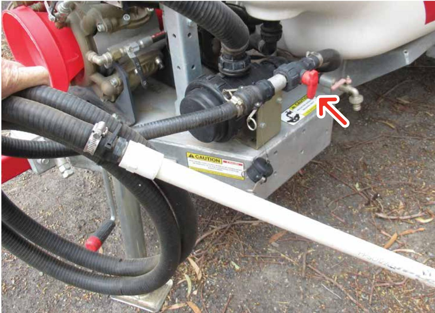
The suction probe has two taps. The first is at the pump which activates the venturi system to create the suction, and the second tap allows the probe to be turned on / off or set to partially open as required.
