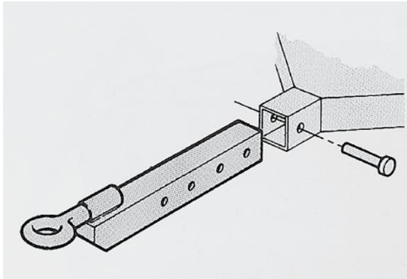
All Cropliner Sprayers are fitted standard with an adjustable length drawbar. It can be used with the tow eye on top or on the bottom.
