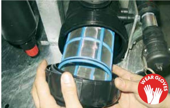
Remove the outer filter screw and bowl
