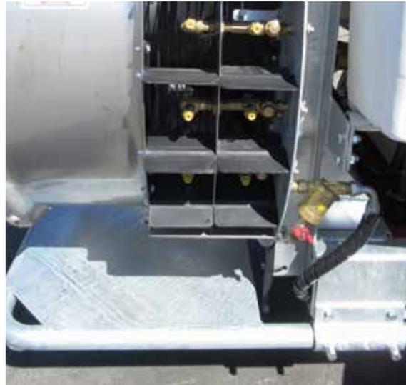
Sprayers using the 1060 fan are fitted with a non-adjustable heavy-duty guard (pictured left).
