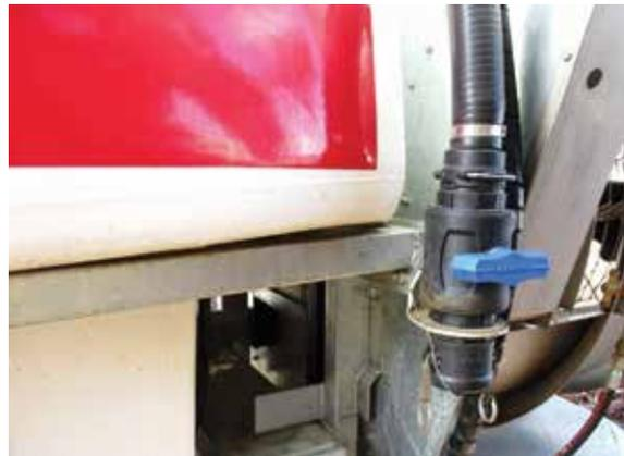
Some operators prefer to fill from a premixed tank, others will prefer to add powders via the basket or concentrate chemical via the probe to a fully or partially filled main tank.
