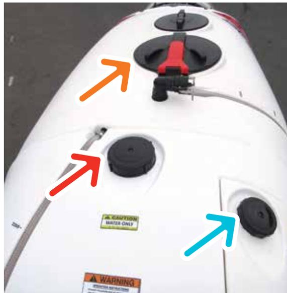
The 15 Litre **Hand-wash** tank is a separate integrated into the flushing tank at the top front left corner of the sprayer (see Blue arrow fill point), FRESH WATER ONLY. See tap outlet below.
