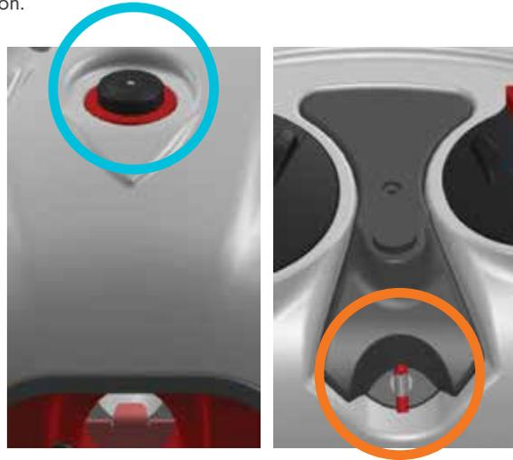
The red 120 Litre freshwater **Flushing** tank is located towards the front of the sprayer. The design is integrated with the main tank and transmission tunnel. (**blue circle** fill point). FRESH WATER ONLY.
