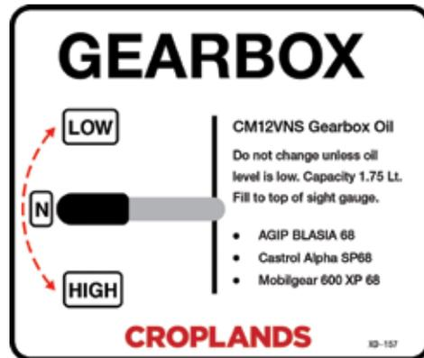
All units are supplied with a lever to engage and disengage the fan.
