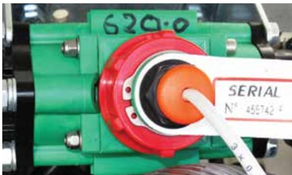
To check / improve the resolution of the flow meter calibration use the below method after having sprayed out a reasonable volume of liquid (the more sprayed the better the resolution);
