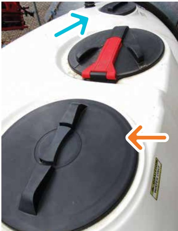
**Do not use this lid as a fill point unless the operator has a purpose-built platform to allow safe access to the lid.**
