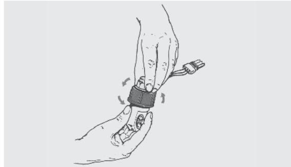
2. Separate the sensor from the Rapid Check unit.
