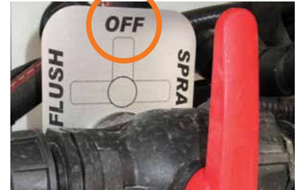
The pump suction valve CLOSED to the main tank
