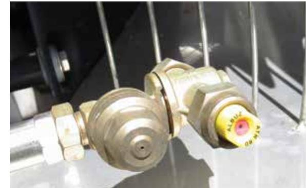
Shown with steel disc & cores plus Albus ATR (yellow) nozzles.
