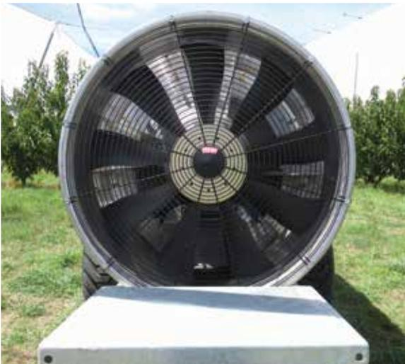
From time to time the incoming air guard may become clogged with leaves etc. Always disengage the fan before removing clogged leaves etc from the guards.
