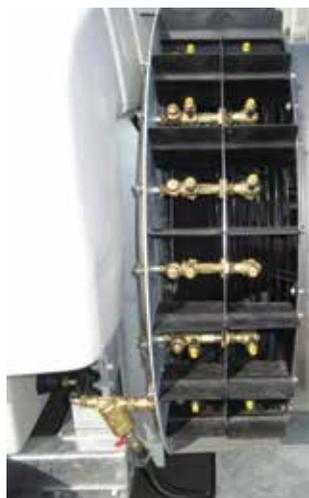
**Fieni 920 DSV Fan, DETAILED NOZZLE PLAN, Albuz ATi Hollow Cone Nozzles.**
