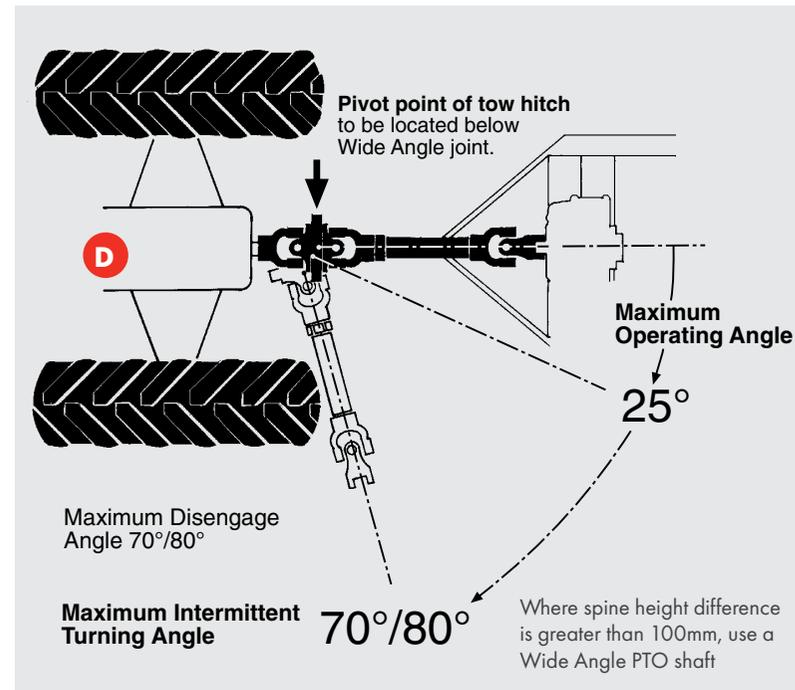
These shafts perform very differently when turning the tractor and sprayer at the end of rows. They must be set-up and operated within the limits outlined.
