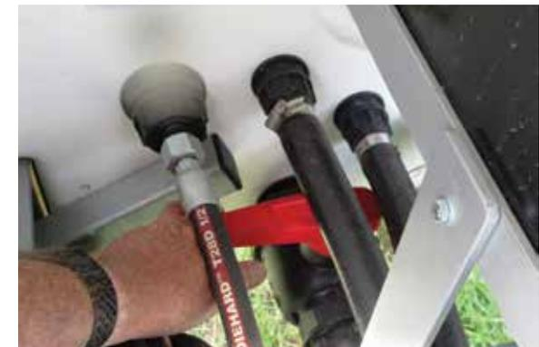
**Drain** completely via the drain valve at the front of the tank. See tap handle in photo below.
