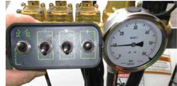
The up position is ON. To activate spraying, flick either or both spray section switches to ON. Adjust the pressure to suit.
