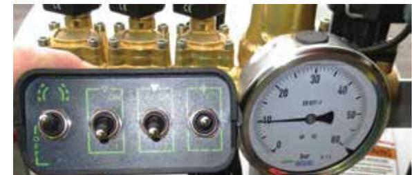
Note: Re this controller, always finish with the master switch in the middle off position (to avoid a flat battery).
