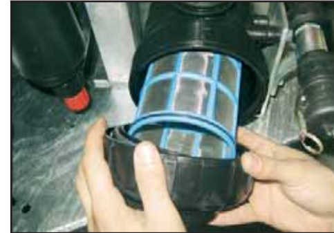
Remove & clean the filter element & components.
