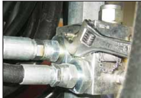
Loosen the lock nut on the PRV.
