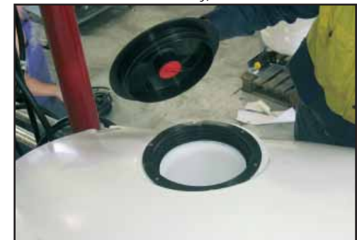
Remove the lid shown to fill the fresh water tank (4000 litre only).
