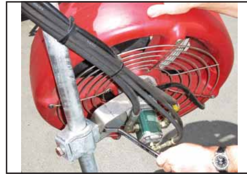
Adjust mount for tilt (upwards or downwards) in relation to canopy.
