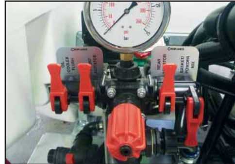
Test the operation of the selector valves.
