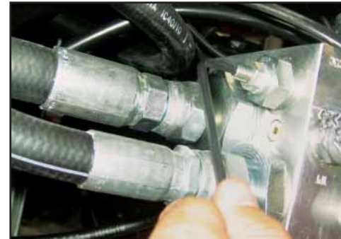
Adjust the PRV with the hex key.
