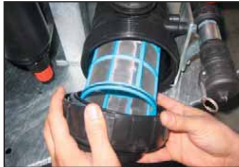
Remove the outer filter screw and bowl.
