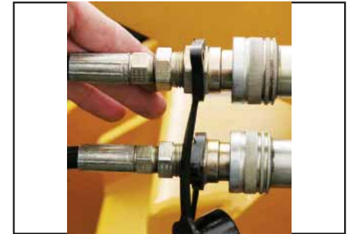
Connect the Tower fold/unfold hoses to the tractor (Fold Tower models only).
