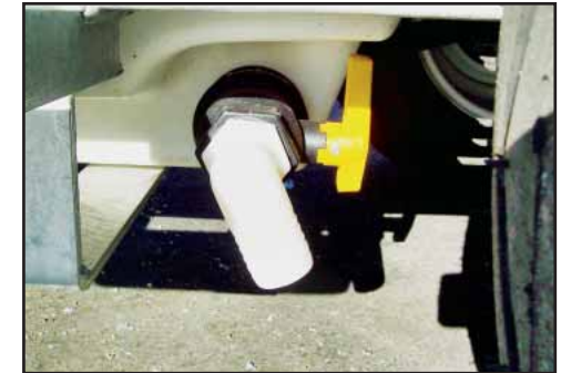
Tank drain valve CLOSED.
