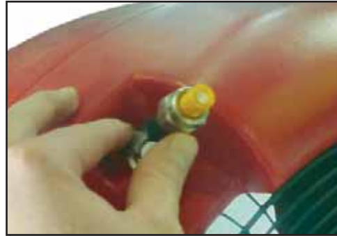
Nozzles adjusted for canopy spraying.
