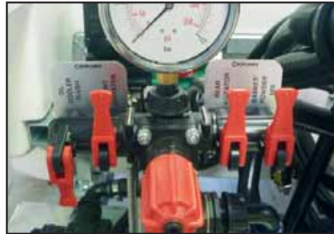
Agitator & mixing basket valves OPEN.
