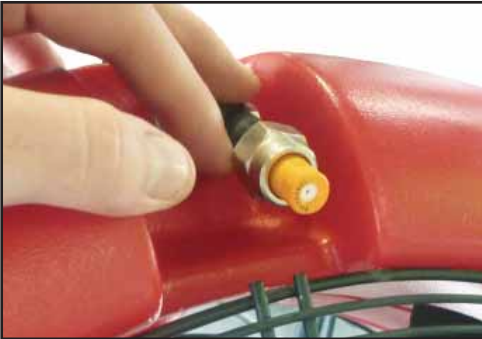
Nozzles adjusted inwards for bunch line applications.
