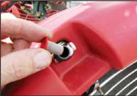
Regularly check and clean nozzle filters (if fitted).
