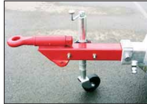
Attach & adjust hitch jack before removing drawbar pin.
