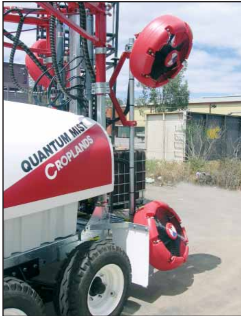
Optional terrace boom allows individual boom arm height adjustment.
