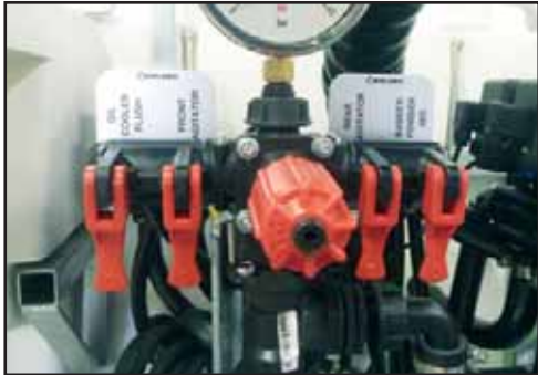
Agitator and mixing basket valves CLOSED.
