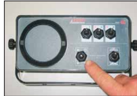
If fitted, test pressure UP/DOWN switch and ensure maximum pressure is 12 bar.
