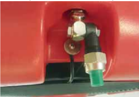
Tighten nozzle swivel to hold setting.
