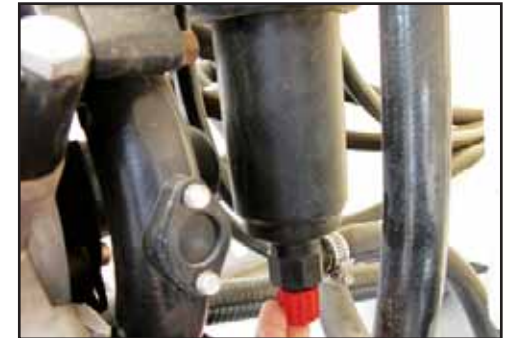
Open & close the filter tap while system is pressurised.
