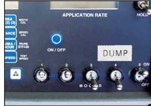
Right & left booms are activated by boom switches 1 & 2. Switch 4 is used to activate the main On/Off dump valve.
