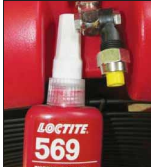
Always use thread sealant Loctite 569 or equivalent when fitting the swivels to the spray ring.
