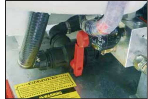
CLOSE the pump suction valve before filter cleaning.
