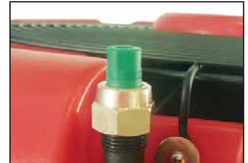
Remove & soak nozzles in Farm Mate cleaner.
