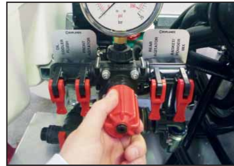
Adjust PRV for Pressure Control.
