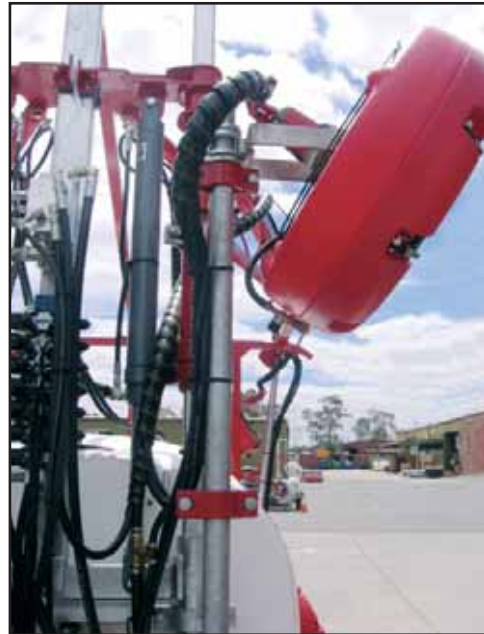
Terrace boom height adjustment hydraulic rams in mid point position.
