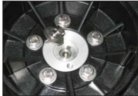
Fit the fan & mounting hub to the drive body shaft
