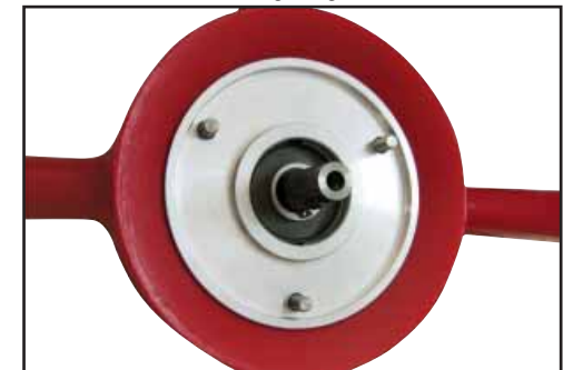
Install the retaining flange (HD-219-20)
