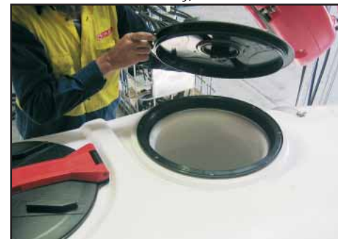
Remove the lid shown to fill the flush tank (4000 litre only).
