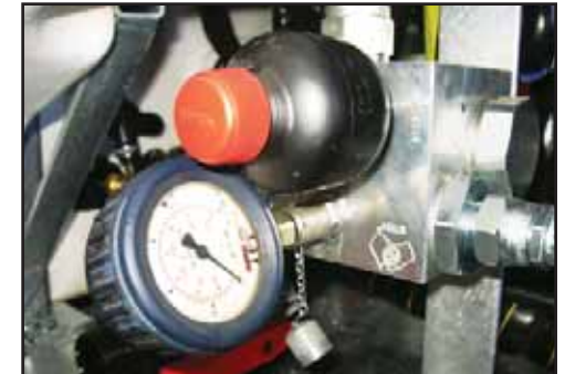
Set maximum pressure on the TPP port to the required pressure.
