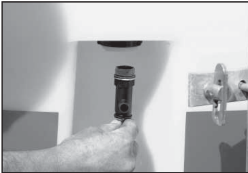
Remove the tap from fresh water tank outlet.
