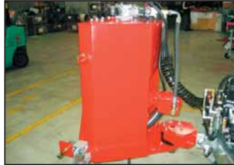
Optional PTO mounted hydraulic supply.
