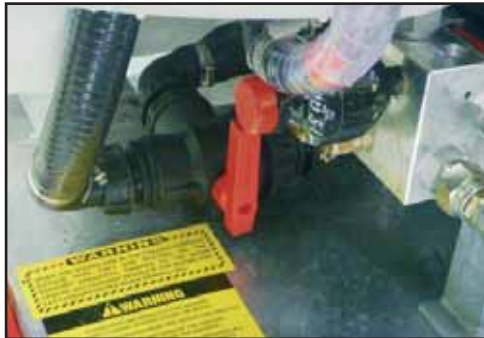
The pump suction valve CLOSED to the main tank.
