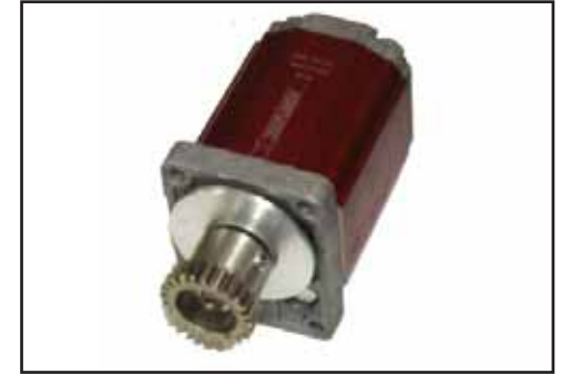
Fit the hydraulic motor to the drive body
