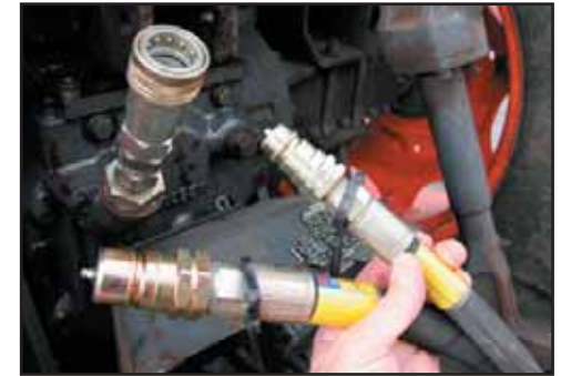
Return fitting installed and ready for hook-up of the return line.
