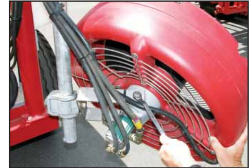
Adjust mount for forward/rearward fan adjustment.
