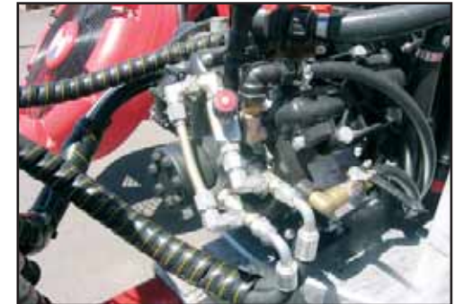
Independent oil supply fitted with hydraulic drive pump.
