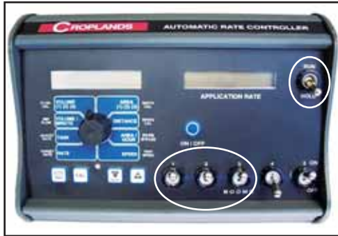
Test RUN/HOLD and LEFT/RIGHT functions.
