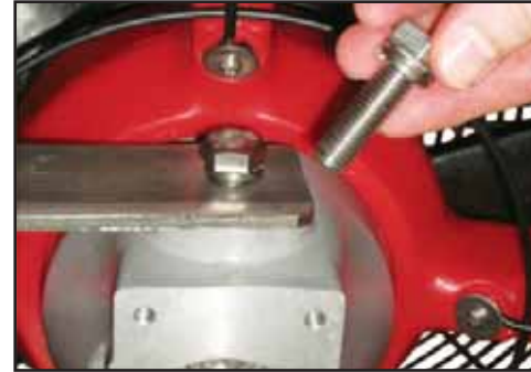
Fit the mounting bracket to the drive body
