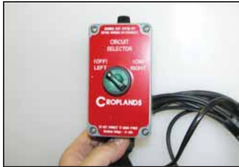
In-cab control switch for fold/unfold and wiring connector.
