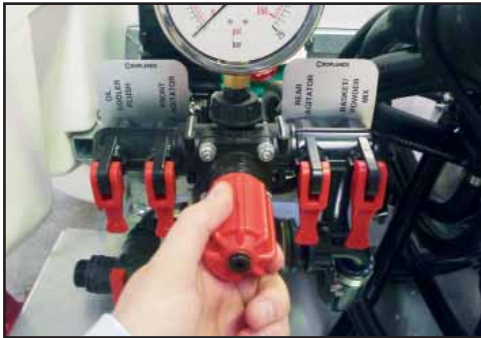
Adjust the sprayer pressure with the pressure-control knob.
