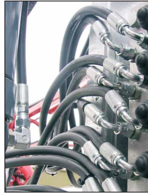
Terrace boom hydraulic manifold with CETOP3 valves.
