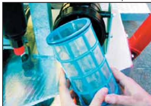
Remove & clean the filter element & components.
