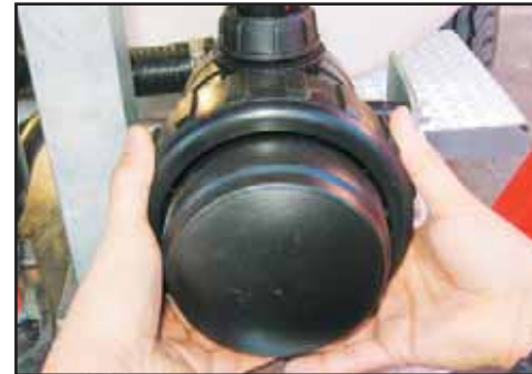
Reassemble and tighten the outer filter screw.
