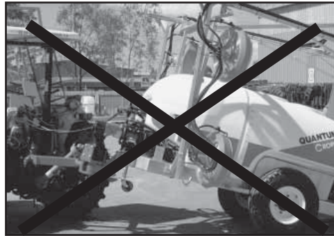
Failure to lock linkage arms may cause damage or injury.
