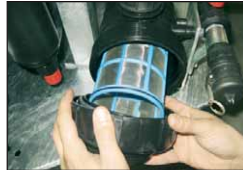
Check suction filter is clean.
