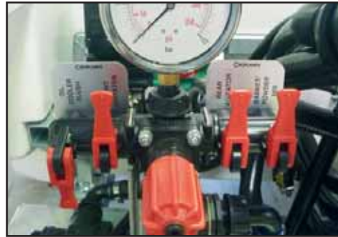
Agitator and mixing basket valves OPEN.
