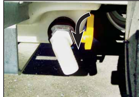
OPEN the Tank drain valve.
