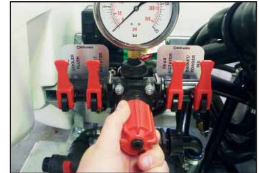
Adjust pressure control knob (PRV) if required.
