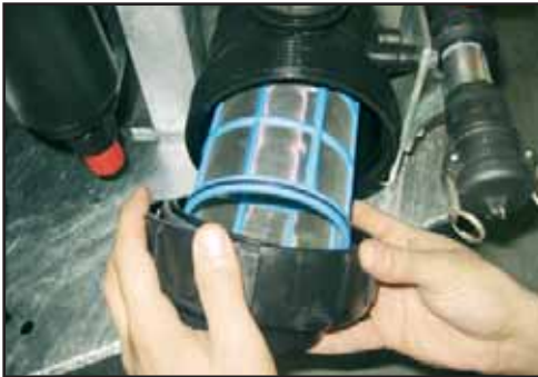
Thoroughly clean the suction filter and reassemble.
