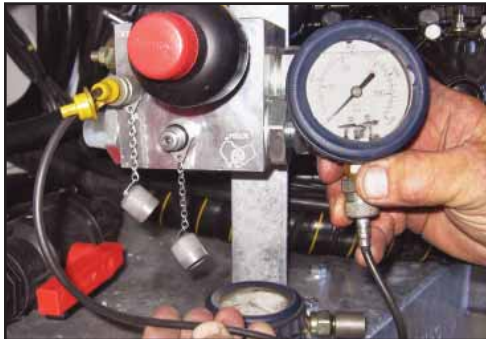
Maximum pressure at TPT (low pressure port) should not exceed 6 BAR (4 BAR during operation).
