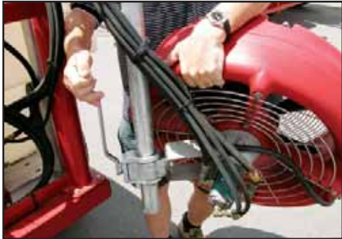
Adjust height of fan on inner/outer tube.
