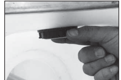
Remove the centre flange from the fresh water tanks.
