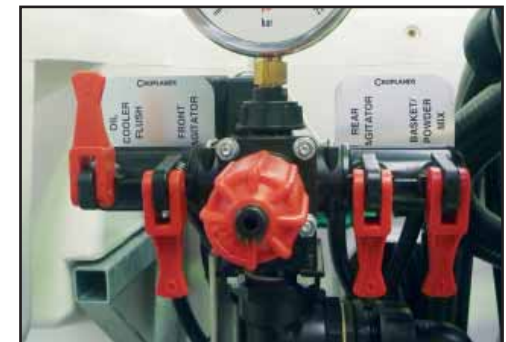
Left hand UCM switch for Heat Exchange Flushing shown in the 'ON' position
