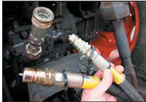
Connect hydraulic hoses to the tractor.
