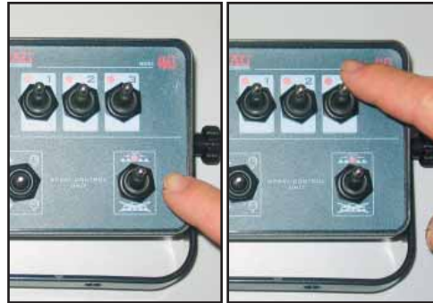
Test master ON/OFF and LEFT/RIGHT functions.
