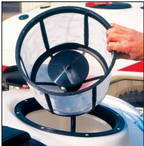
The mixing basket assists adding chemicals to the tank.
