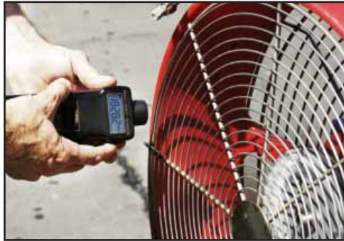
Check fan speed using an RPM meter.
