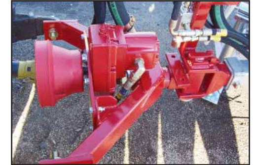
Optional self-contained hydraulic system & self-tracking drawbar.
