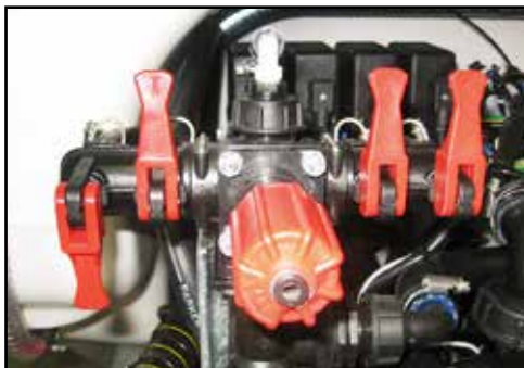
Agitator and mixing basket valves OPEN.
