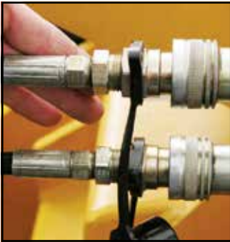
Plug boom-fold hydraulic hoses into tractor remotes.
