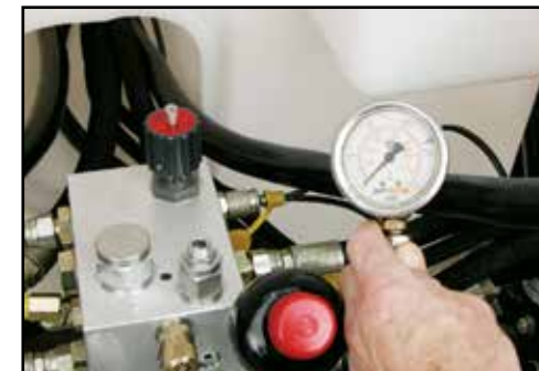
Set maximum pressure on the PPT port to ...
