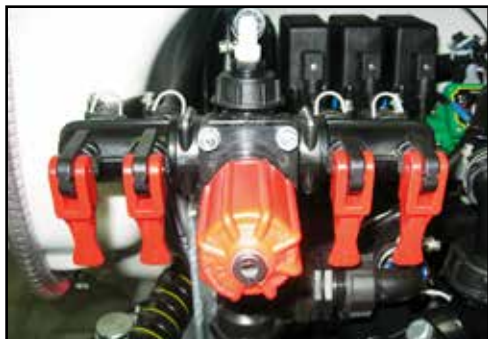
Agitator and mixing basket valves CLOSED.
