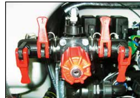
Agitator valves OPEN & mixing basket valve CLOSED.
