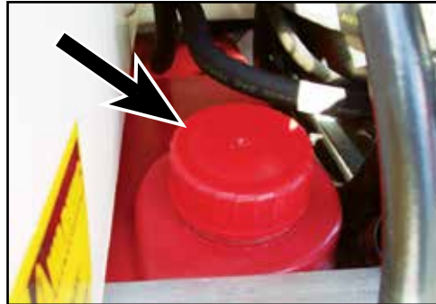
Remove the lid shown to fill the flushing tank.
