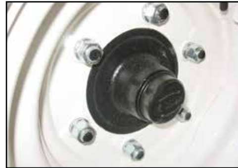
Grease wheel hubs.
