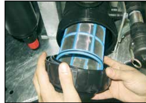
Remove & clean the filter element & components.
