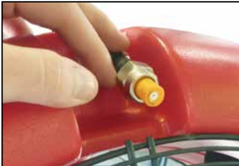
Nozzles adjusted inwards for bunch line applications.
