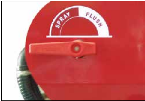
Pump suction valve OPEN for liquid from the main tank.
