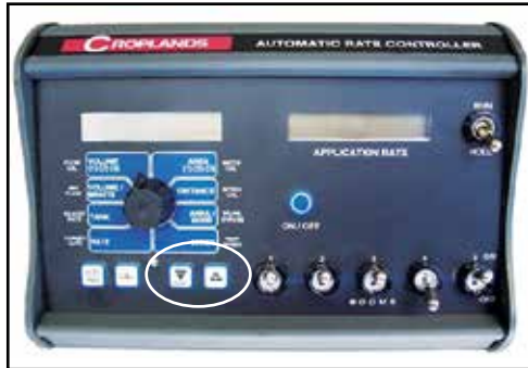
Test the pressure UP/DOWN with console in Manual Mode (MT3405).
