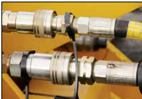
Hook up the hydraulic supply & return lines to the tractor.
