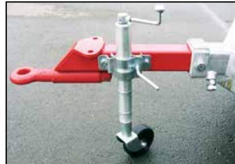
Hitch fitted in the lower position.
