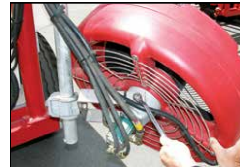
Adjust mount for forward/rearward fan adjustment.
