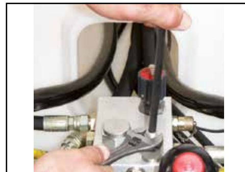
Loosen the lock-nut on the PRV and adjust with hex key
