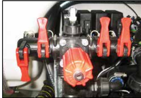
Agitator & mixing basket valves OPEN .
