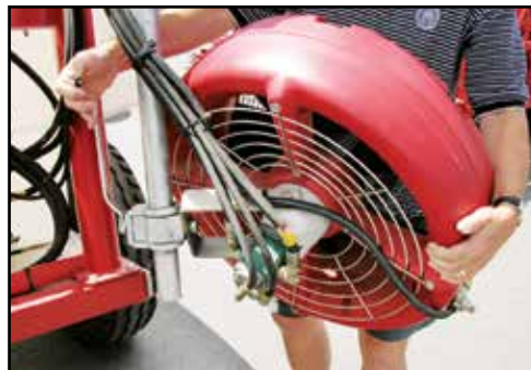
Spin mount to move fan closer to canopy, and to allow tilt adjustment.
