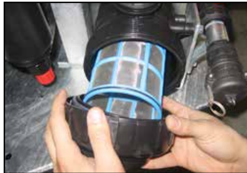
Remove the outer filter screw and bowl.
