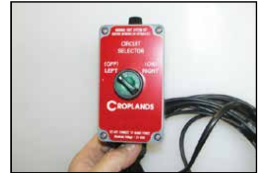
In-cab control switch for fold/unfold and wiring connector.
