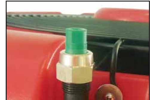
Remove & soak nozzles in Farm Mate cleaner.
