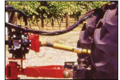
Grease the PTO shaft.
