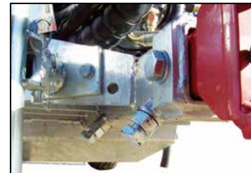
Loosen the bolts and locking nuts that hold the hitch.
