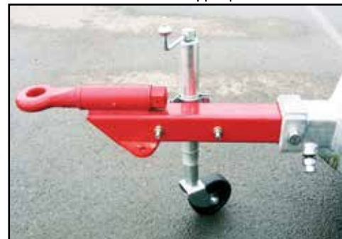
Hitch fitted in the upper position.
