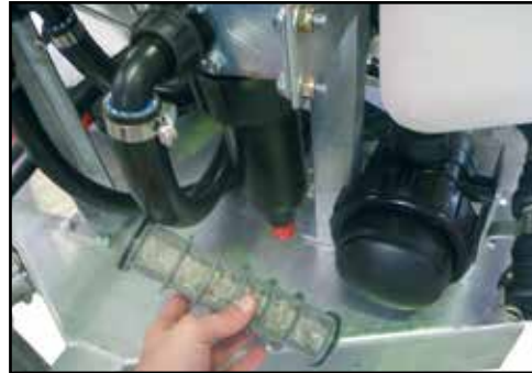
Clean pressure line filter regularly.
