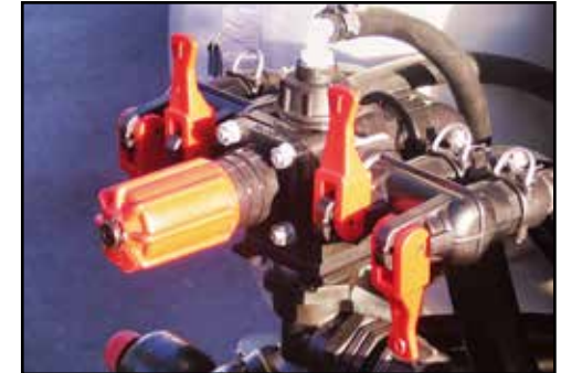
Front and rear tank agitator valves in ON position.
