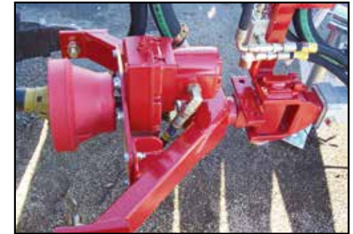
Optional self-contained hydraulic system & self-tracking drawbar.
