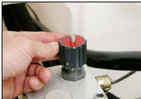
Ensure the manual pressure/flow valve is wound-out fully.
