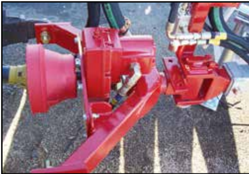
Grease all swivel drawbar grease points.
