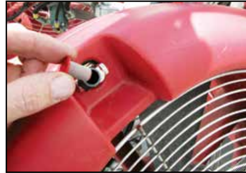
Regularly clean nozzle filters (if fitted).
