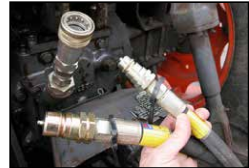
Connect hydraulic hoses to the tractor.
