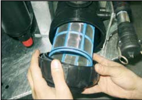
Thoroughly clean the suction filter and reassemble.
