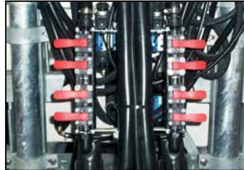
Individual spray heads can be turned ON or OFF.
