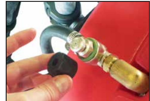
Fan head nozzles can be turned On or Off.
