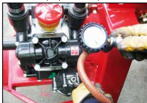
Check pump air chamber pressure.
