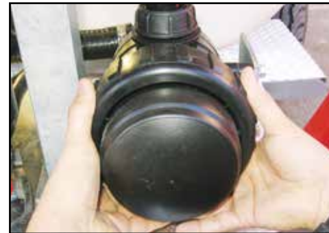
Reassemble and tighten the outer filter screw.
