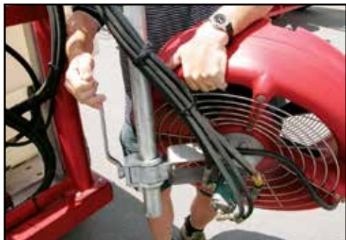
Adjust height of fan on inner/outer tube.
