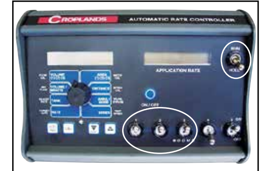
Test RUN/HOLD and LEFT/RIGHT functions.
