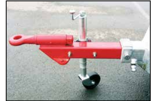
Attach & adjust hitch jack before removing drawbar pin.
