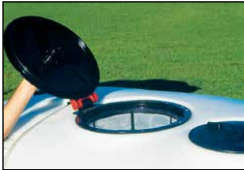
Open the lid & fill main tank using the basket filter.
