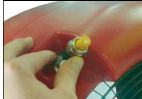
Nozzles adjusted for canopy spraying.
