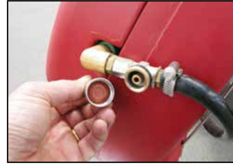
Remove & clean non-drip diaphragms regularly.
