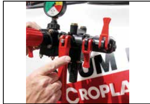
Test the LEFT/RIGHT operator of the selector taps.
