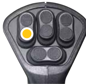
Section L is turned on/off with SW4
