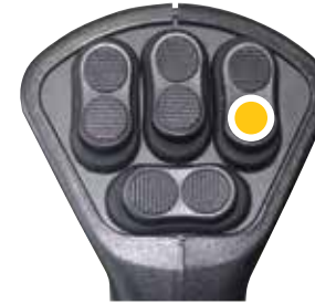
Section R is turned on/off with SW5
