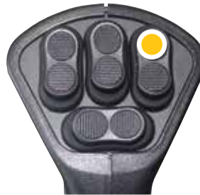
Section RR is turned on/off with SW3
