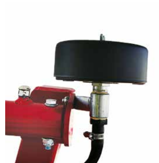
Compressor Air Filter (shown below on sprayer)
