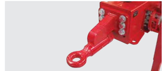
The front drawbar hitch tongue is height adjustable
