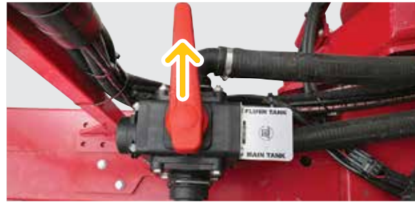
Rotate the front Tank Selection valve to "Flush Tank" position
