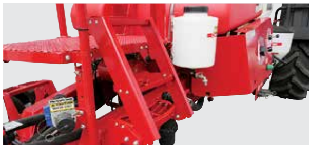
Fold-up the steps on each side at the front of the Sprayer before proceeding to spray
