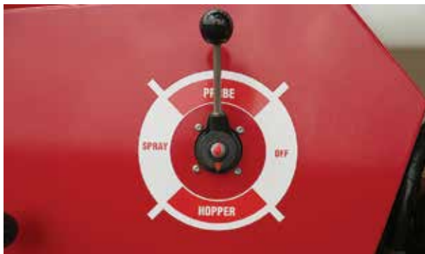
Rotate the Pressure Valve to "Hopper" position
