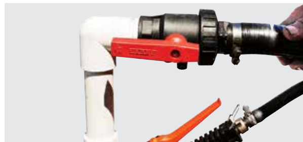
Open Probe valve to transfer mixture to spray tank
