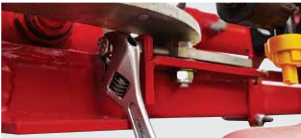
Loosen the lock-nut, then, adjust the adjusting bolt to position the plate to the desired position
