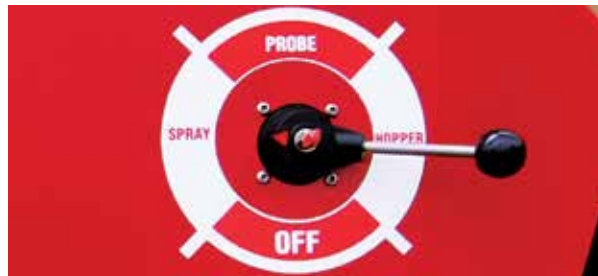
Rotate the Pressure Valve to "Spray" position
