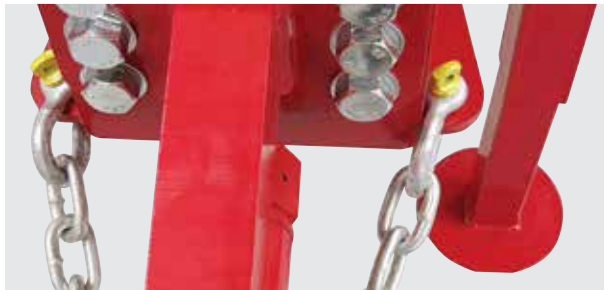
The transport safety chain must be fitted
