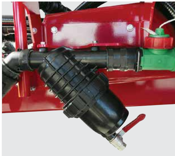
Bottom-Fill Filter (shown below on sprayer)
