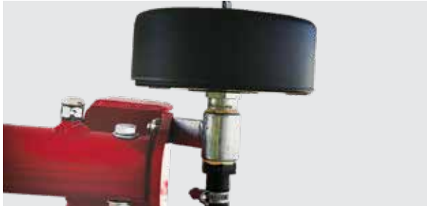
Clean the compressor air filter regularly
