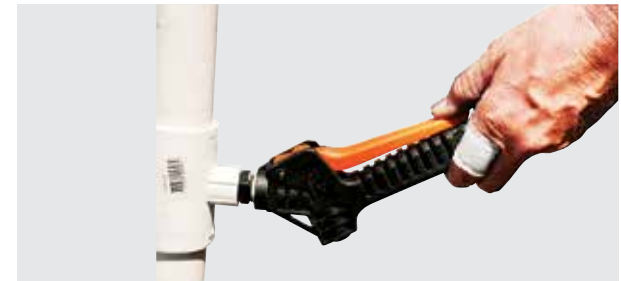
Open Probe valve to transfer mixture to spray tank
