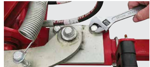
Loosen the holding bolts (2 shown) of the wing locking plate
