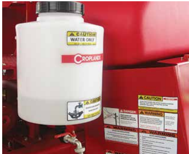
Fresh Water Tank: Fill Cap & Tap
