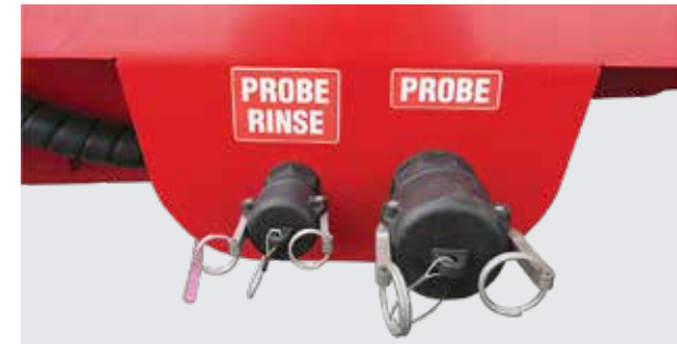
Connect the Probe Rinse & Probe" hoses
