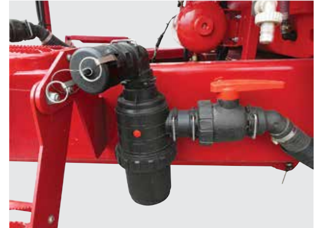
Main Tank Fill Connector (2")
