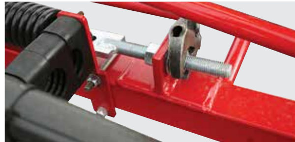
Adjust the breakaway arm spring pressure to the desired setting to hold the wing section firmly
