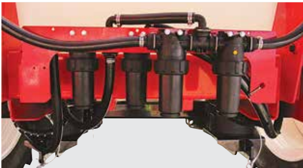
Clean the main pressure filters regularly
