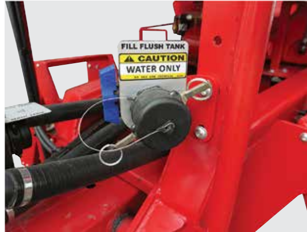
Flush Tank Fill Connector (2")
