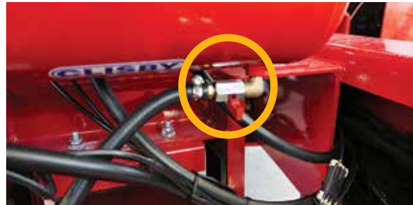
Drain moisture from the compressor tank regularly
