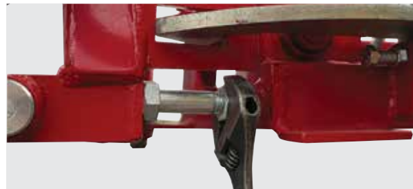
Unlock the bolt stopper lock-nut
