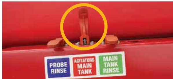
Open the Agitators Main Tank valve
