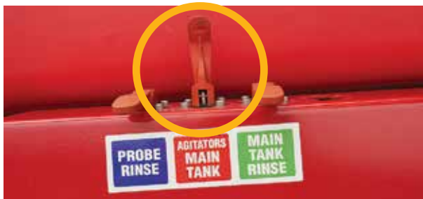
Open the "Agitators Main Tank" valve before adding chemical
