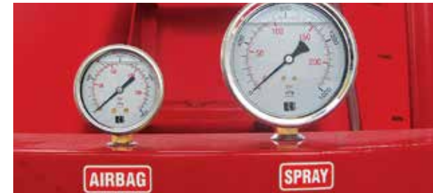
Airbag & Spray Pressure Gauges located on the front of the Sprayer
