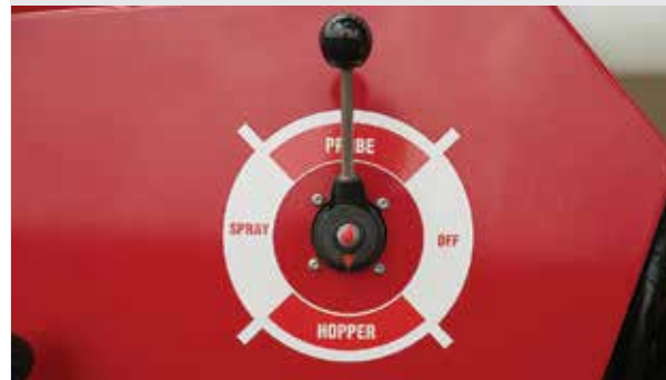
Rotate the Fill valve to "Hopper" position
