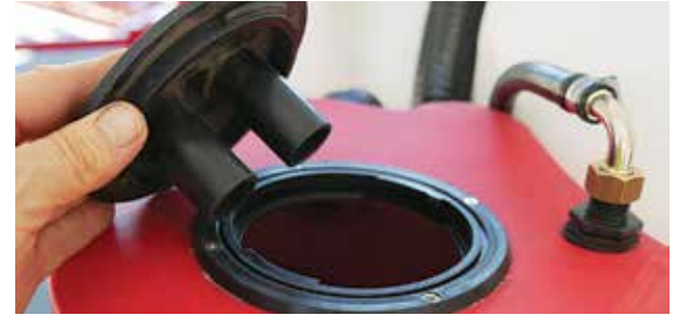
Open the Flush tank lids for inspection
