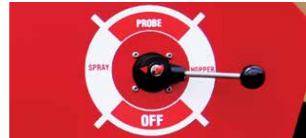
Rotate the Pressure valve to "Spray" position
