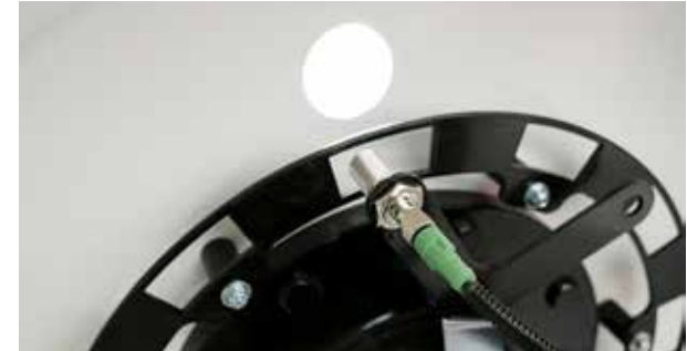
Check the spacing between the speed sensor & magnets
