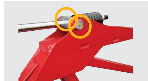
Grease the upper inner-boom hydraulic ram hinges
