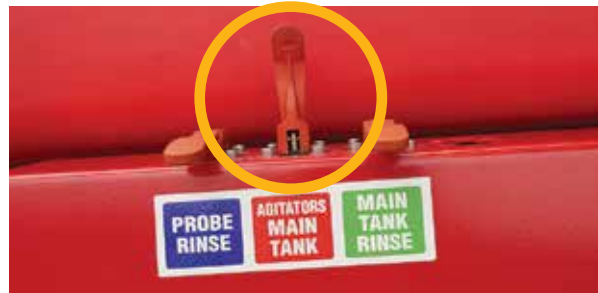
Open the "Agitators Main Tank valve before adding chemical
