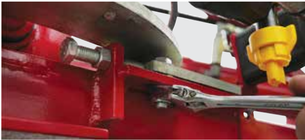
Loosen the holding bolts (1 shown) of the wing locking plate
