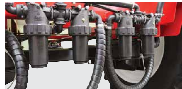
Remove & clean all pressure filters
