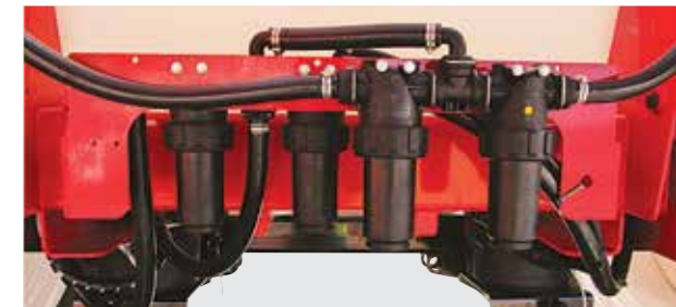
Clean the pressure filters
