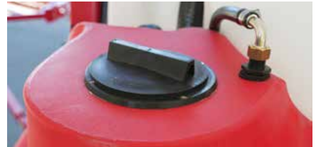
Replace Flush tank lids after inspection
