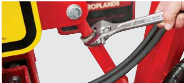
Unlock the lock-nut on the turnbuckle
