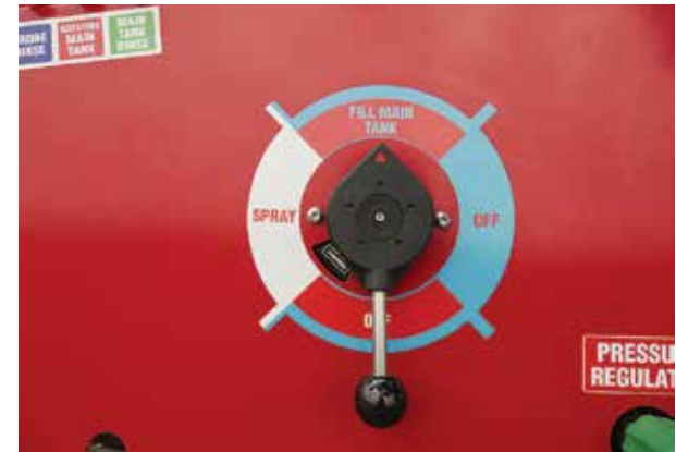
Rotate the Fill valve to "Fill Main Tank" position
