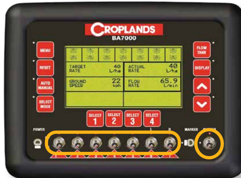
Switch Boom Sections On & Off several times.
