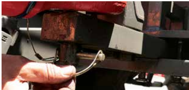
Ensure the drawbar pin is locked-in
