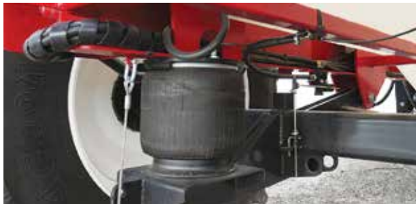
Air axle & levelling valve with adjustable linkage
