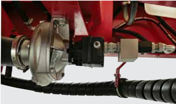
Hydraulically driven Hypro centrifugal pump
