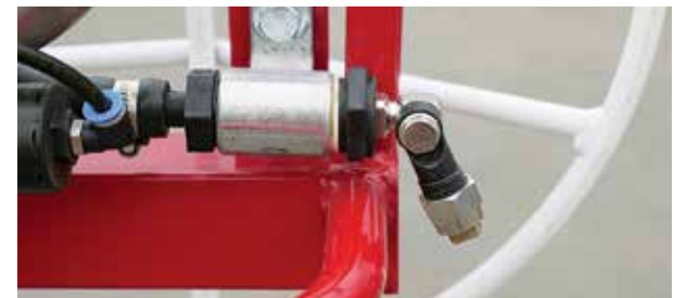
Check Fenceline nozzles are working correctly
