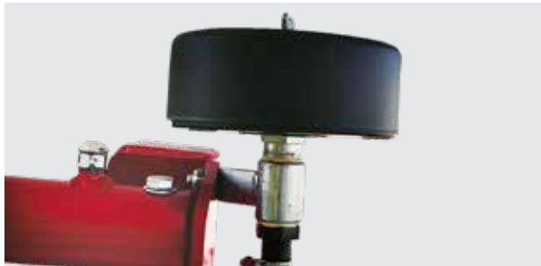
Clean the compressor air filter regularly
