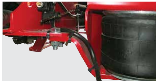
The ARDS drawbar inflatable airbag mechanism
