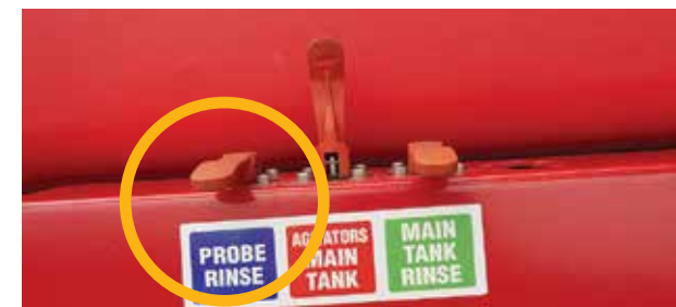
Close the Probe Rinse valve on the main control panel
