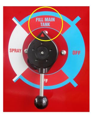
Note; position of the Pressure valve is not critical whilst filling, but best to be OFF unless required.
