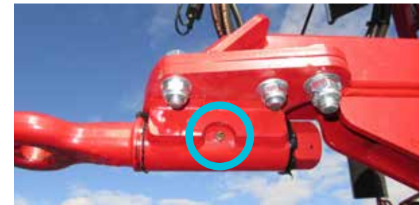
Grease all swivel drawbar grease points
