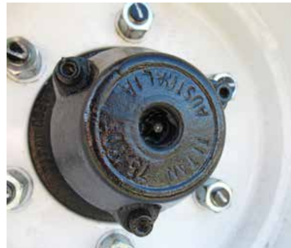
Grease all swivel drawbar grease points
