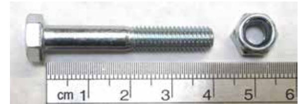
Shear pin bolt requires 20mm of plain shank
