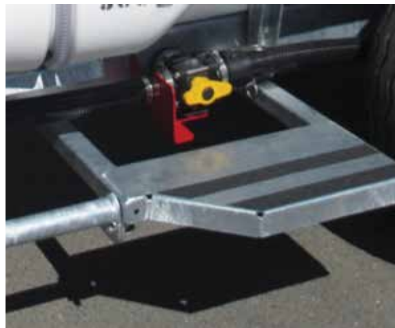
Access to the top of a spray tank is best effected by using a purpose built platform.
