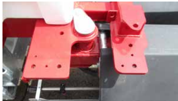
Shear pin bolt requires 20mm of plain shank
