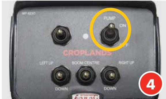
4. Engage the pump, by turning the pump switch to ON (up)
