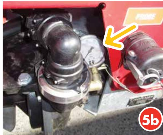
6. Adjust the Spray pressure via the pressure regulator
