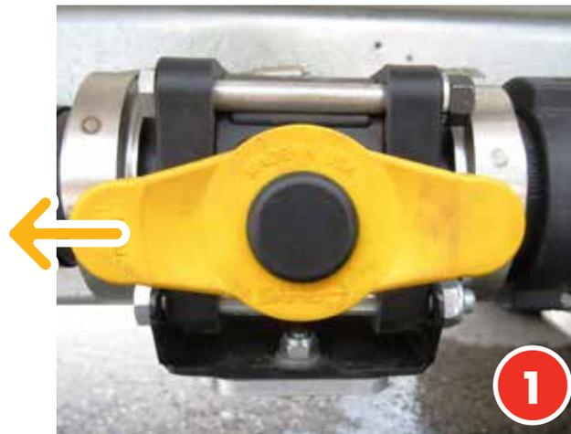
1. Main tank ball valve set to the Pump / Spraying (left)
