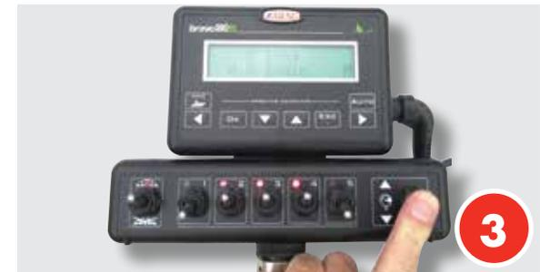
3. Go to the Arag controller, turn on the master on/off switch and all three boom sections. Hold the manual pressure switch up for 5 seconds to set maximum pressure with all boom sections spraying. Note the photo above is of a 5 section controller (using middle 3 sections).
