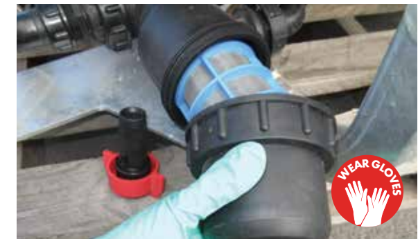
Remove the outer filter screw and bowl
