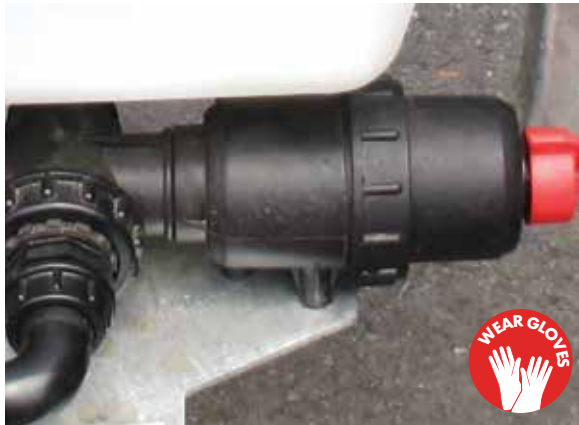
Reassemble and tighten the outer filter screw.
