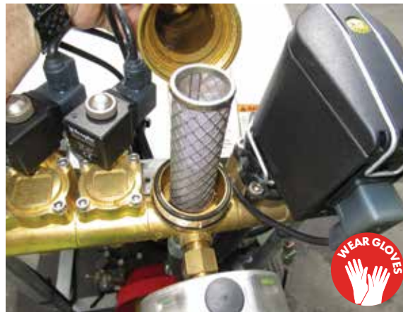
Open & close the filter tap while system is pressurised
