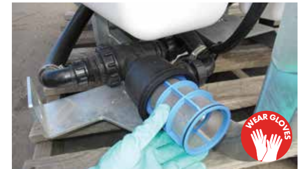
Remove & clean the filter element & components
