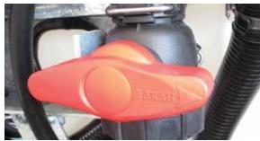
• Unscrew the outer filter ring and remove the bowl, then remove the (blue 50-mesh) filter. Thoroughly clean the filter and reassemble - checking the o-ring.
