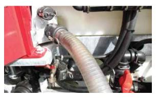
The fill line is equipped with a one-way valve to prevent splashback.
