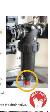
• Remember to re-tighten the drain valve.
