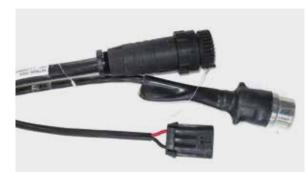
A new installation of the Fusion controller will require a direct power connection to the tractor battery.
